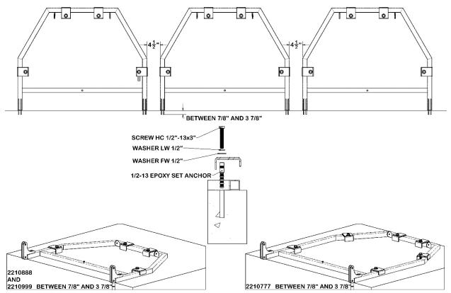
• If you are assembling several units into a continuous wall, bases must be spaced 4 1/2" from each other.
